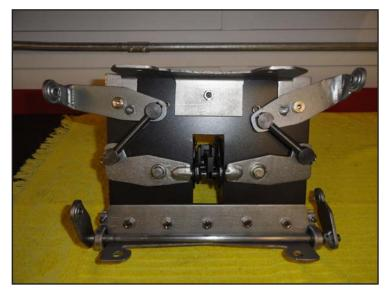
The thing that makes this all possible is the Heim joints. The Heim joint is a ball and housing that rotates bi-laterally as shown below. We don't care about the threaded part, so the female ones work just a little better than the
