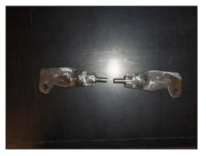
They must be opposing each other and have the rod protruding upward on the proper side. The protruding rod must be 3/4" and be cleanly welded so that the entire 3/4" can be used. Now that you are ready to weld, clamp the rod down to the table as well as the pivot so its positioned correctly and go for it!
