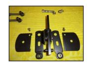
Since this is a solid design, we can accomodate both with minor adjustments. So let's make the tower bracket to fill that 3-1/4" by 1-1/2" hole you labored over in the top plate. Using 10 gauge steel. Cut out two pieces that are 3 inches by 4 inches. The hardest part of this procedure is trying to get the center hole at the proper height for the lower mechanism to meet up properly. There are two issues we are concerned with here. One is proper
