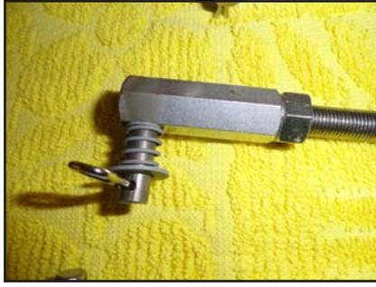
Weld the 5/16" rod by placing weld inside that end of the coupling nut. Pretty solid way to hold the rod in. Sometimes things just work out! Now, cut three pieces of 3/8"-24 all thread that is as follows:
