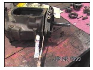
Put a couple of bolts in the center section, and leave the heads out about 1/2"- no more than this to keep the tranny's main shaft bearing pins in place. Work gasket sealer in the edges here using a screwdriver.
