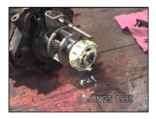
Slide the sun/planets/clutch on while holding the shift rod in the sun gear's fork groove. It will take three hands for this one. Don't forget to put the reverse lockout rod in it's hole first. You will have to use heavy grease to glue the clutch pins in place. Apply sealer to the case mating surface now.
