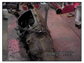
Remove any bolts, and carefully slide the rear case onto the unit. Help here is good. Have the helper turn the yoke to get the gears lined up as it goes together. The linkage rod slides into the hole with the spring. make sure the notch is facing down on the rod, and the spring is in the center of the hole. It you hear a clutch pin drop and hit the case, start over again.
