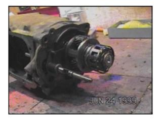
The rear case removed. This is the center section, and contains the rear bearing, linkage, solenoid mount, and gear assy for the overdrive. The transmission's main shaft is part of this unit, and it takes the place of the rear tranny case on a non-OD unit.
