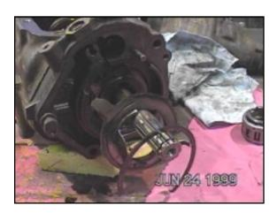
Remove the big snap ring to release the splash guard and linkage face plate. The solenoid locking gear and slide block resides in here.
