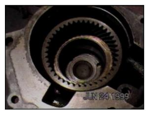
This is looking into the clutch hub and ring gear. There is a stepped section that's rough in the first part of the center's machined smooth section. Don't panic. This is normal, and it helps the clutch pins slide in during reassembly.
