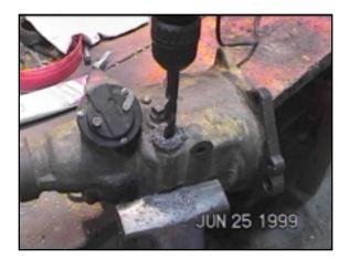
This unit didn't have oil drain plugs. Typical 1970's Save-A-Buck thinking. The castings are there, so we drilled them for a 1/4" pipe plug fitting. The choice is yours. Do it now, or lay underneath with a turkey baste bulb later while trying to suck out the old oil!
