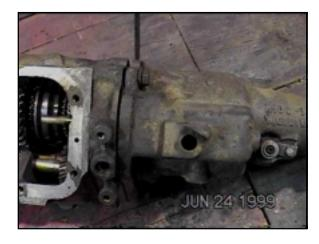
>>> DON'T let the case next to the transmission come apart! Note in the picture where the crack is starting. If the center section slides out, the bearing pins in the main shaft of the transmission will fall out! Hours of extra work if they do!!
