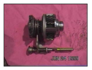
This is the shift rod in overdrive position. The groove in the sun gear lets the planet cage spin past.
