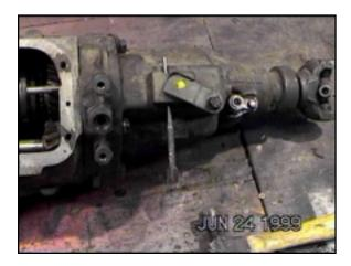
The first step is to remove the freewheel clutch lockout taper pin. If you forget, the case won't come apart due to the linkage inside. Remove the lockout lever too.
