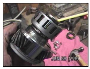
Assemble the clutch onto the planet set. It's a bit tricky to get the big U-Clip snapped on again. Having help is great.
