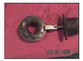
In direct, the solenoid lets the block slide out. The sun is released and tries to spin in the planets. This causes a lockup of the planet set, and the sun, planets, and ring gear spin as a unit. The shift rod lets the sun slide back into the planet case so it locks solid for direct.
