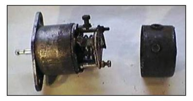
The overdrive solenoid with the cover removed. When powered, the shaft puts pressure on locking dogs until engine torque is released, then the locking dogs engage the planet set case, and the ring gear then rotates 27% faster than the input shaft. The large terminal is the (S)olenoid line, and the (I)gnition terminal has a short to ground when the shaft is in the engaged position.
