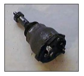
This centrifical switch (Borg Warner calls it a governor) is a key part of the O/D setup. It switches to ground at 27 MPH, and releases at 21 MPH. They put thought into the speeds at which it operates. If you are in 2nd, it will shift up at 27 MPH. You let up on the gas, then step on it again for 2nd over. When you turn a corner, it will automatically downshift back to 2nd as you make the turn. It's GREAT!!
