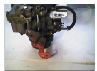
This is the passing gear microswitch on my old carburetor. I didn't use the circuit with the built up 400 small block. It puts out way too much torque for the tranny gears to survive the slamming of very many passing gear kickdowns. I use the release switch and ease it down a gear instead.
