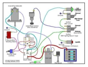
This is a diagram for wiring a split shift control setup for your T-85N transmission. This can be used for one you've bought outright and have no original circuits for, or modifying the one you already have. The DPDT relay is a **D**ouble **P**ole **D**ouble Throw relay. Radio Shack carries them. The passing gear lockout switch is for when you want to run flat out without it dropping out of top gear.
