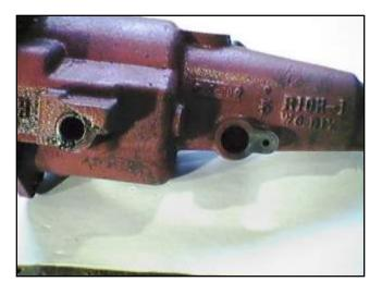
This is a Borg Warner T-85N case with the componants removed. The hole on the left is for the freewheel clutch lockout. The right hole is for the speedometer. These photos are of my spare overdrive unit.
